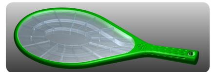
Cobalt's photorealistic rendering shows the internal grid structure of the racquet.
