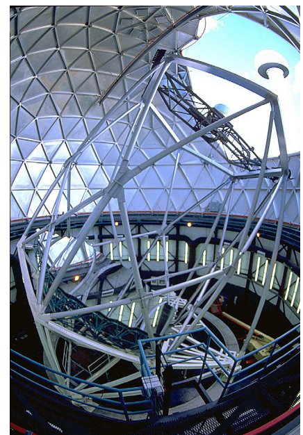
One of the largest optical telescopes in the world, the Hobby-Eberly has an effective aperture of 10 meters and a 78-square meter, hexagonal mirror array made from 91 segments.
